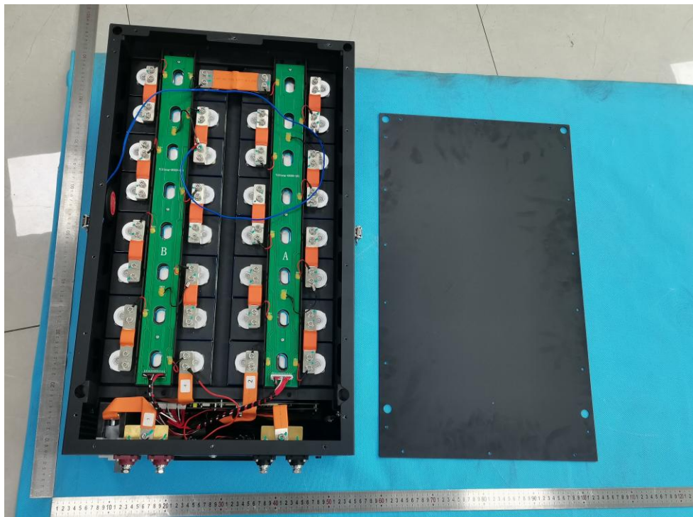
Figure 4 Interior view of battery Pack
